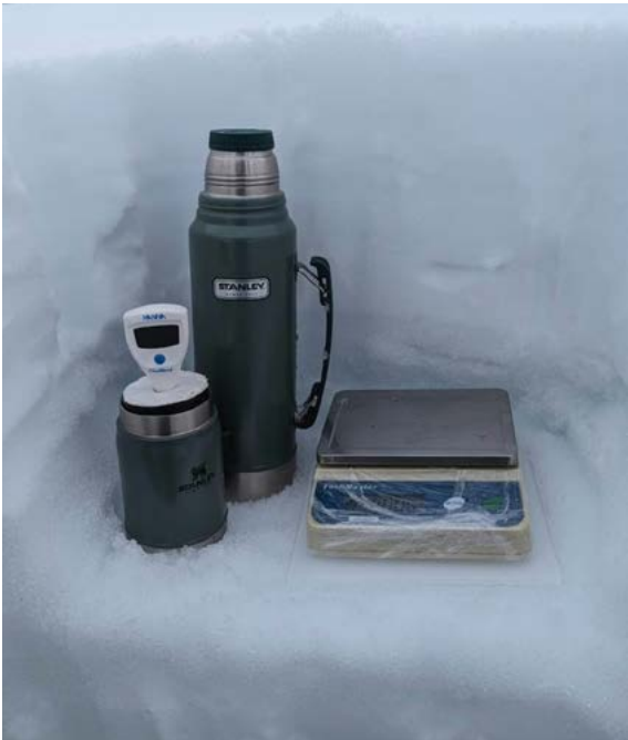
This is how a field research protocol comes to life – through expertise, hard work, and determination. Carlo Marin, group leader of the Mountain Cryosphere research group, together with his colleagues, developed a protocol for using a calorimeter to measure the amount of liquid water in snow and improve predictions of peak snowmelt. Much of the testing was carried out in Val Senales/Schnalstal as part of the Snowtinel project, and the protocol was published in open-source form.
