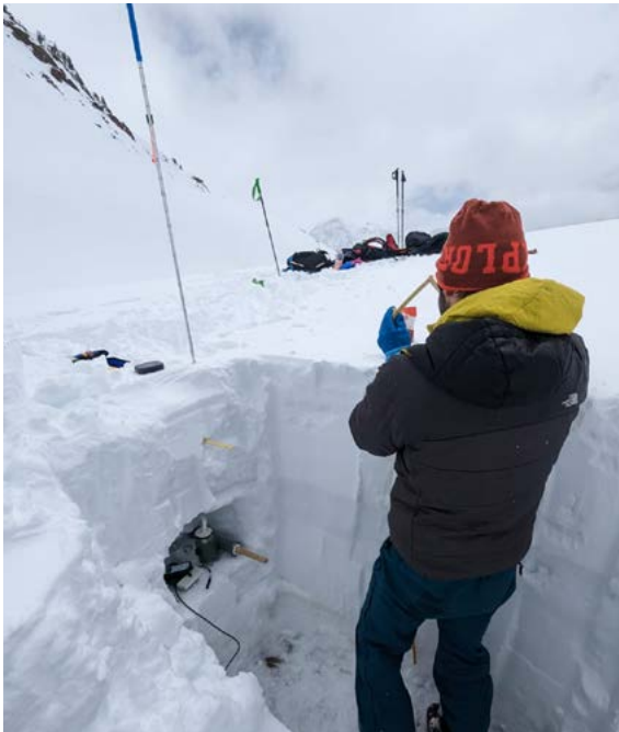
This is how a field research protocol comes to life – through expertise, hard work, and determination. Carlo Marin, group leader of the Mountain Cryosphere research group, together with his colleagues, developed a protocol for using a calorimeter to measure the amount of liquid water in snow and improve predictions of peak snowmelt. Much of the testing was carried out in Val Senales/Schnalstal as part of the Snowtinel project, and the protocol was published in open-source form.
