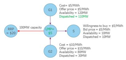
Both generator 1 and 2 are solar generators, and the dispatch interval is in the middle of the day. As a result, both generators are capable of generating a combined output of 200MW, absent of transmission congestion. The introduction of a storage unit, S, means that 10MW more generation is dispatched, all of which is from generator 1 as it is the cheapest and still has sufficient capacity. Less renewable generation is spilt.
