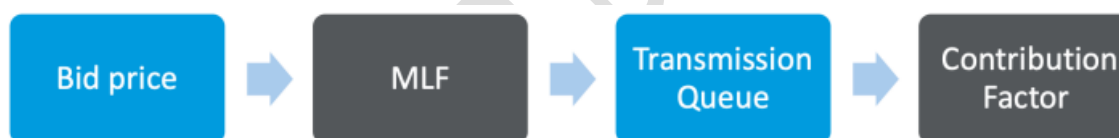
Figure 3 Proposed placement of the queue in the NEMDE dispatch algorithm
