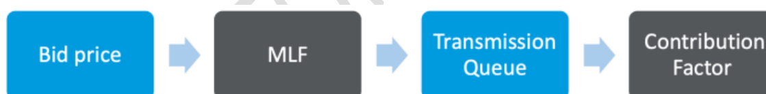
Figure 1 Proposed placement of the queue in the NEMDE dispatch algorithm
