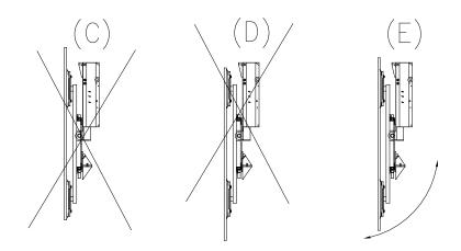
Check that all suckers on the surface are clean and have full contact and, if necessary, press on or align a sucker that is not making contact until it is in the right position. If this is not done, a vacuum cannot build up and the DSMH2-12V can therefore not lift the material. Set the rotary suction switch to ON.
