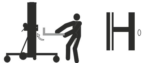
3. Adjust the forks width and check the fitting for each attaching pin.
