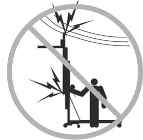
Keep away from the machine if it contacts electrical power lines. Personnel must not touch or operate the machine until power lines are shut off.
