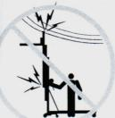
Keep away from the machine if it contacts energized power lines. Personnel must not touch or operate the machine until power lines are shut off.
