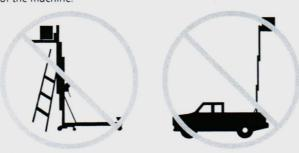
Do not use the machine on a moving or mobile surface or vehicle.
