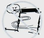
Do not leave a load raised when windy conditions may occur unless the machine(s) are properly guywired.
