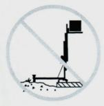
Prior to use, check the work area for drop-offs, holes, bumps, debris, unstable or slippery surfaces or other possible hazardous conditions.
