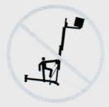
Do not operate the machine in strong or gusty winds. Increasing the load surface area will decrease machine stability in windy conditions.
