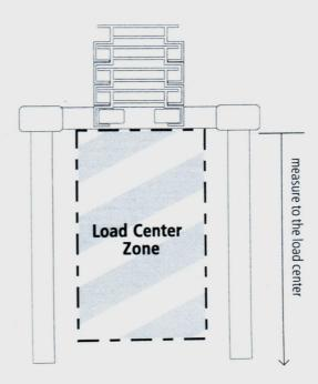
See the chart on the next page for maximum load centers for standard forks, adjustable forks and flat forks.
