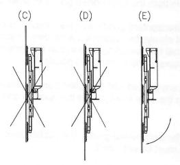
Check that all suckers on the surface are clean and have full contact and, if necessary, press on or align a sucker that is not making contact until it is in the correct position. If this is not done, a vacuum cannot build up and the DSMH4-24V can therefore not lift the material. Set the suction/release valves to the suction position using the remote control.
