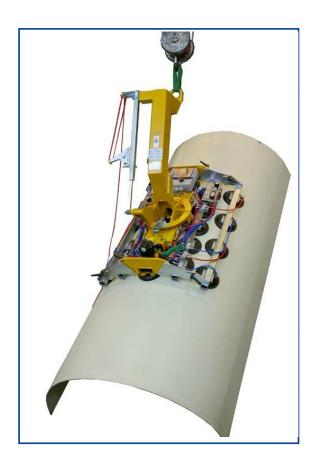
for lifting and transporting of of convex and concave curved materials
