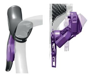
Press the right shift paddle to move the rear derailleur outwards. Press and hold the paddle for multiple shifting.
