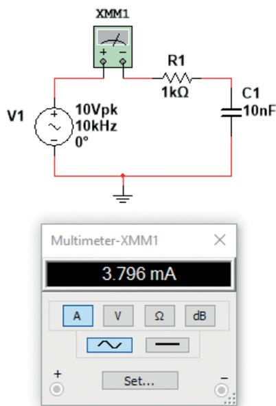
$$V_{\text{eff}} = 10 V_{\text{picco}} / \sqrt{2} = 7,07 \text{ V}$$
