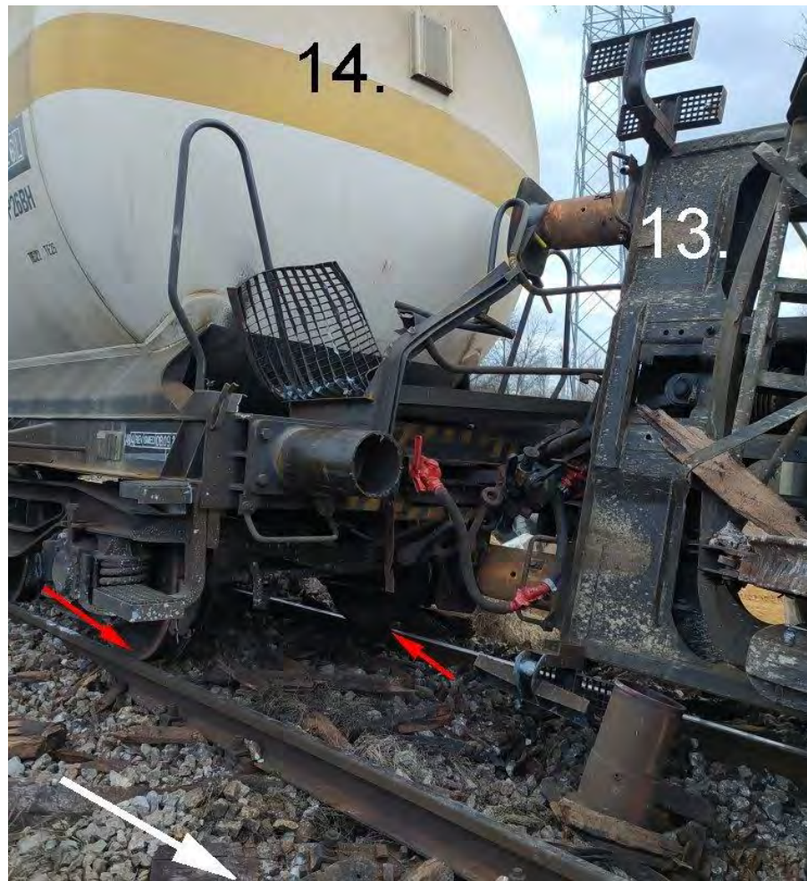
Figure 4.2.1.13: The condition found between the thirteenth and the fourteenth wagon
