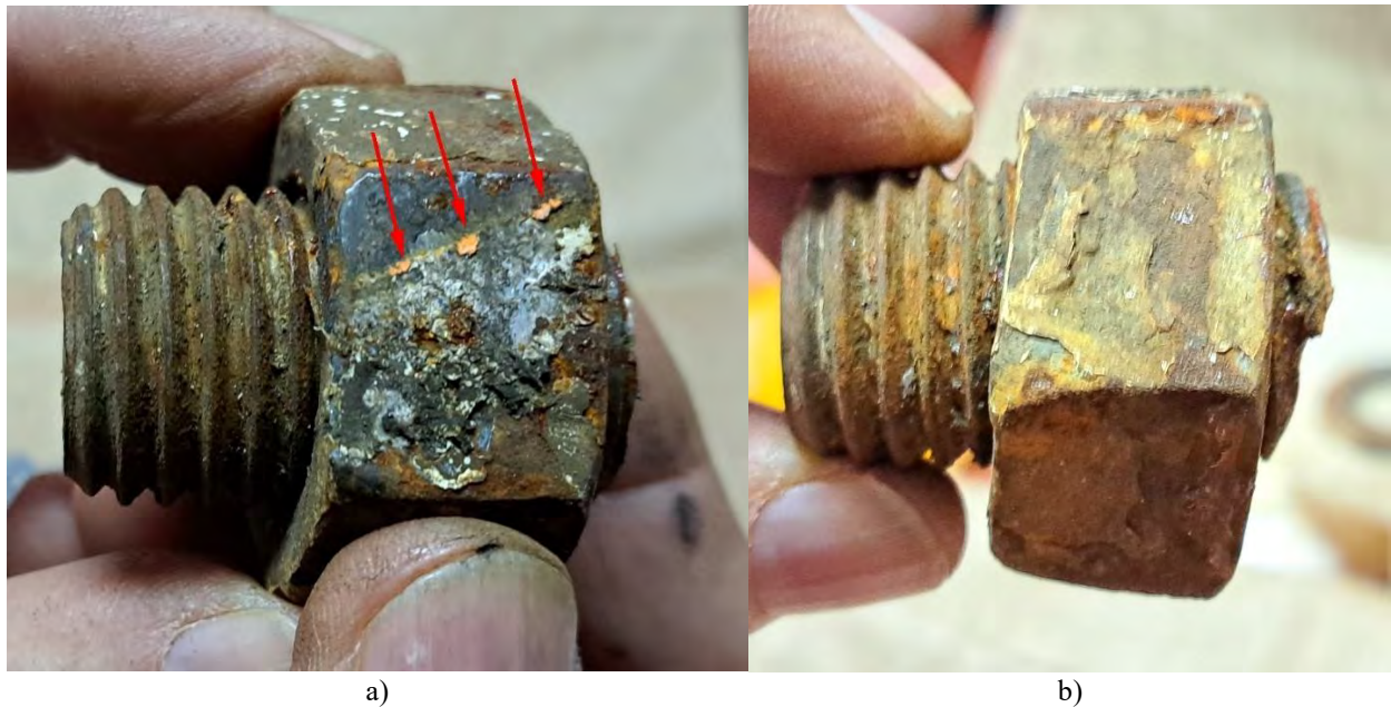
Figure 4.2.1.11: The appearance of the found severed screws
