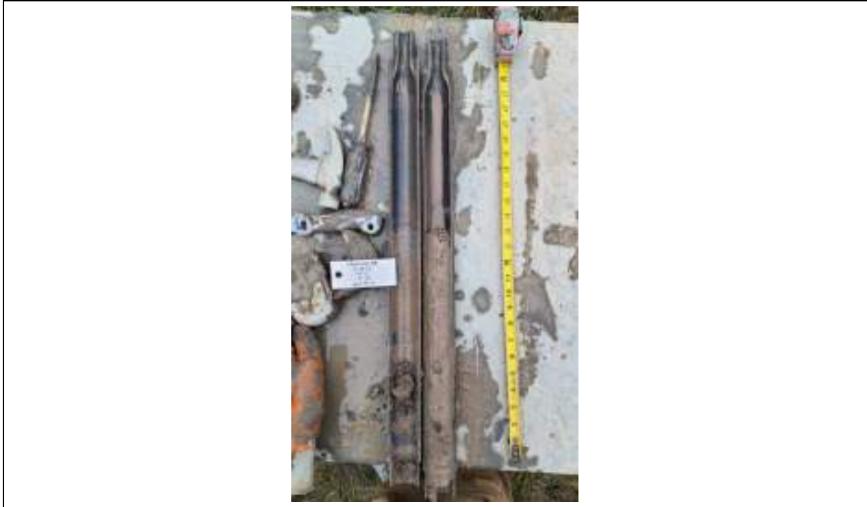
Figure 4-4 Till deposit sample from borehole TF-05-23 (SS-23, 25.91 – 26.52 m)
