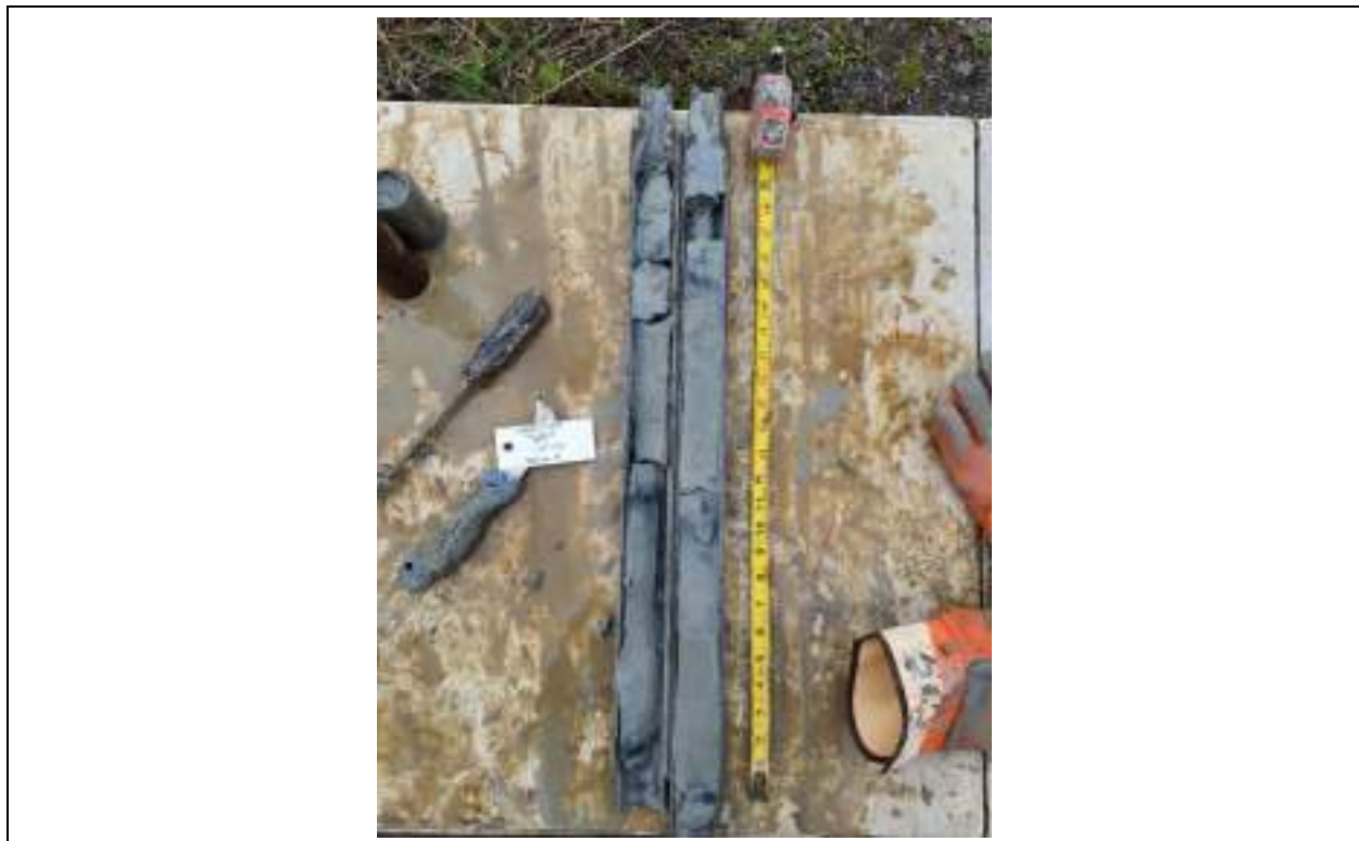
Figure 4-1 Clay deposit sample from borehole TF-06-23 (SS-07, 3.81 - 4.42 m)
