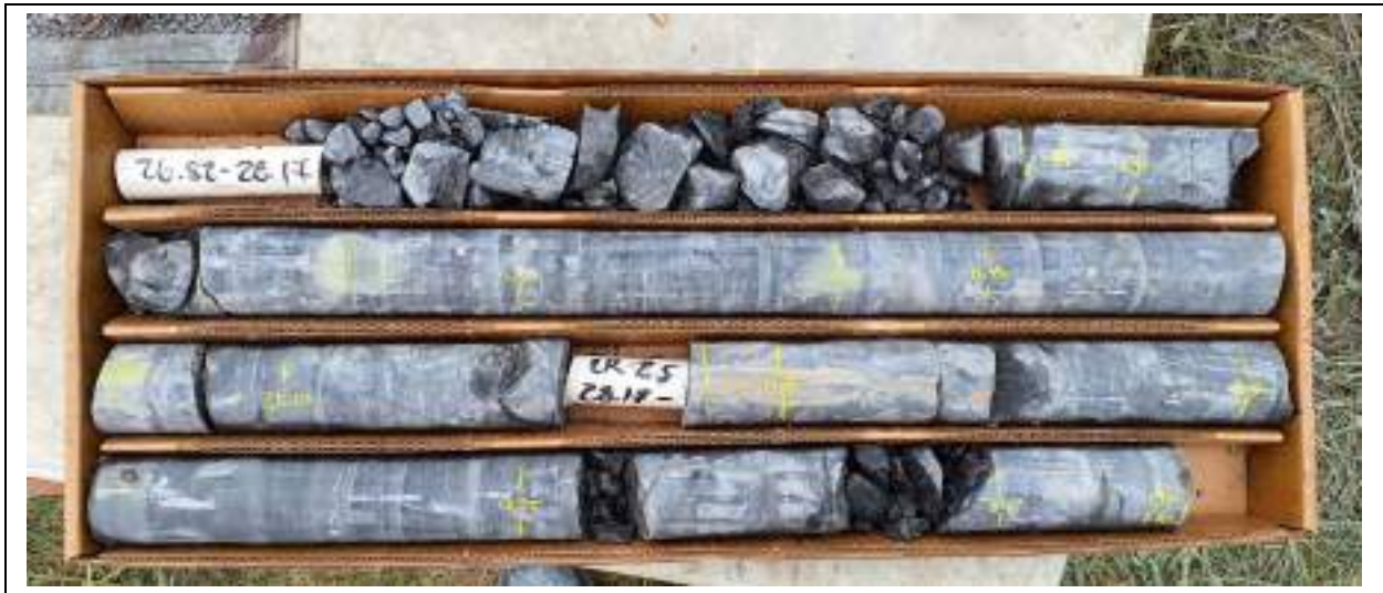
Figure 4-5 Calcareous shale bedrock sample from borehole TF-05-23 (CR-24 & CR-25, 26.82 – 29.10 m)
