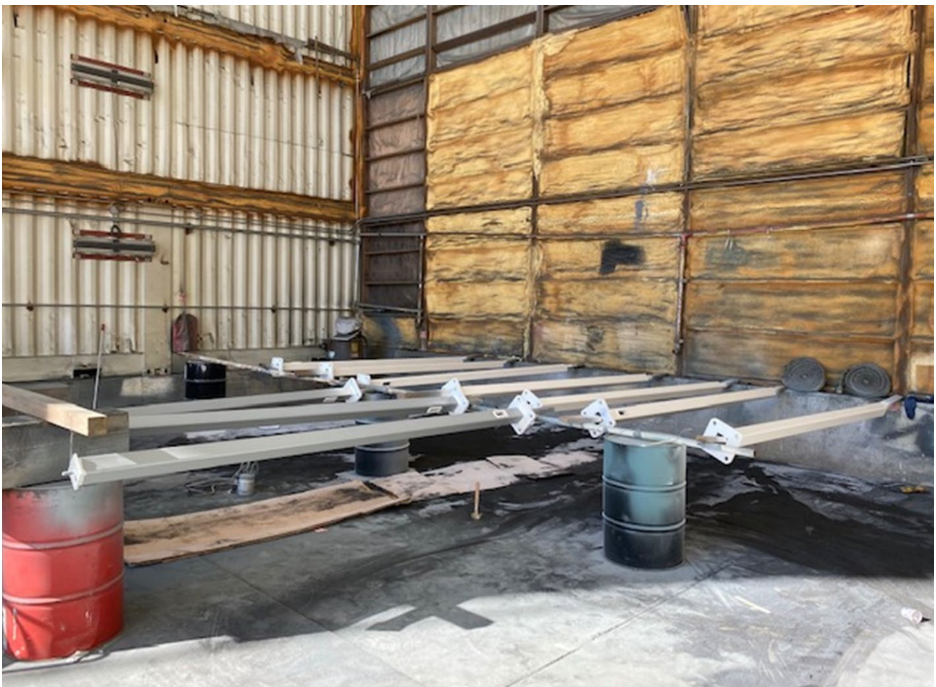
Modified Lamp Posts Receiving Final Coating of Marine-Grade Paint
