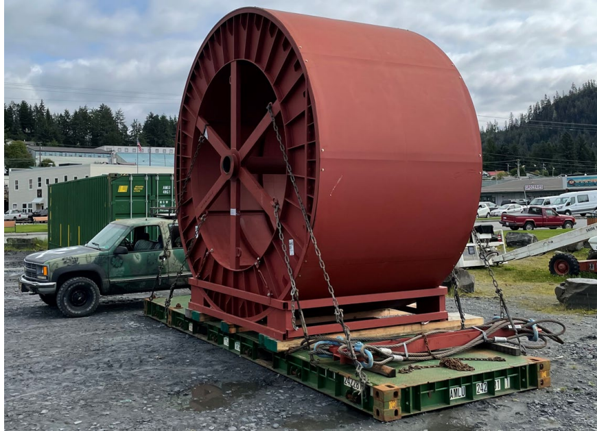
75,000 lb. Spool of Spare Submarine Cable
