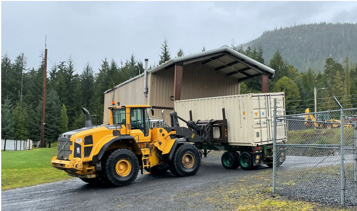
38,000 lb. capacity Loader/Forklift picking Container of Spare Cable Parts
