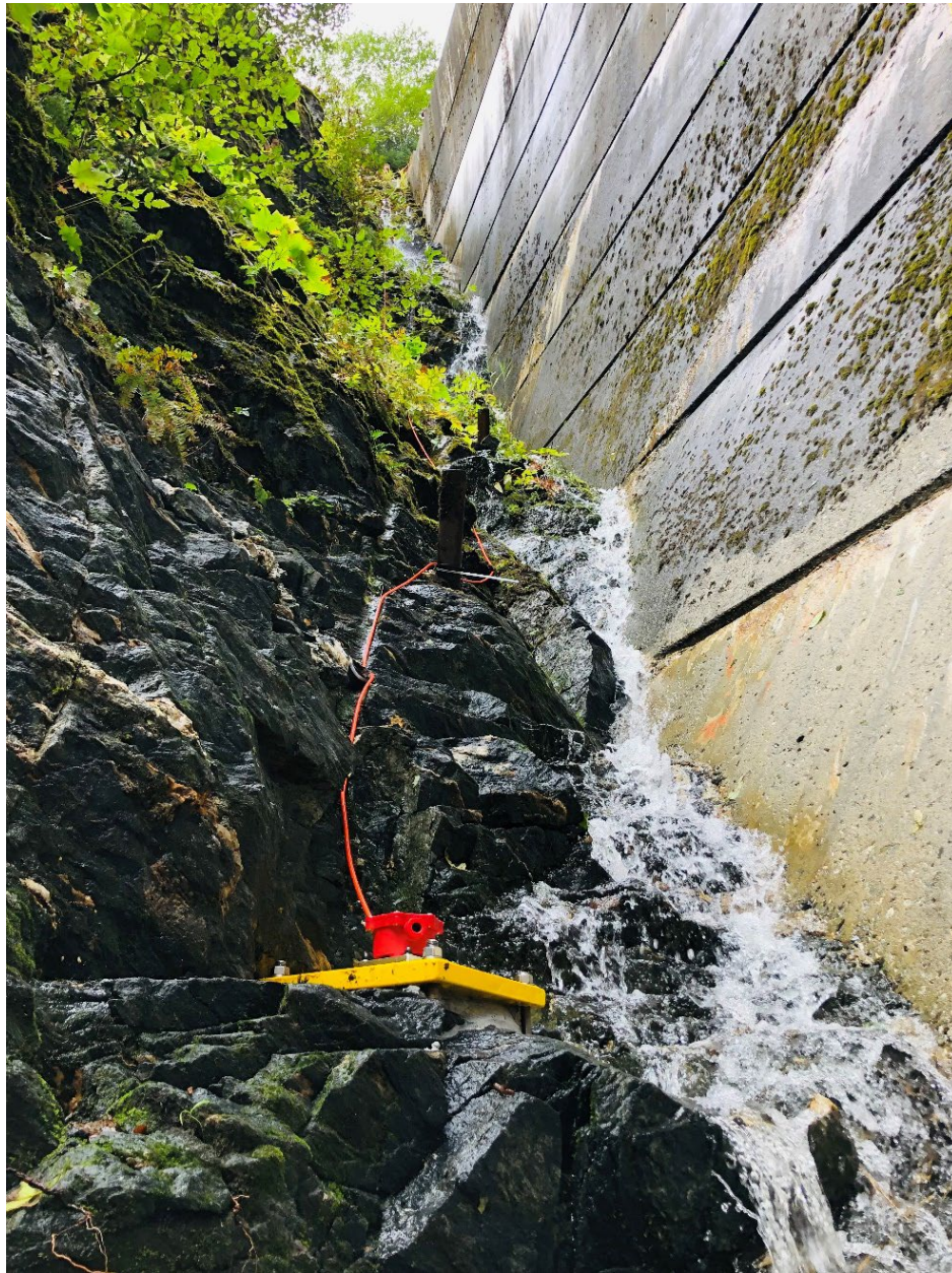
Dam Foundation Vibration Monitoring Geophone
