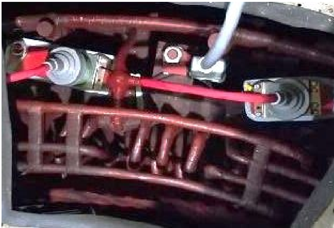
Connection to Coil with Glyptal paint
