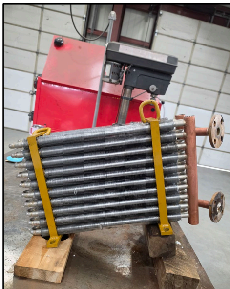
(far left) Photo of patched oil cooler [bottom]
