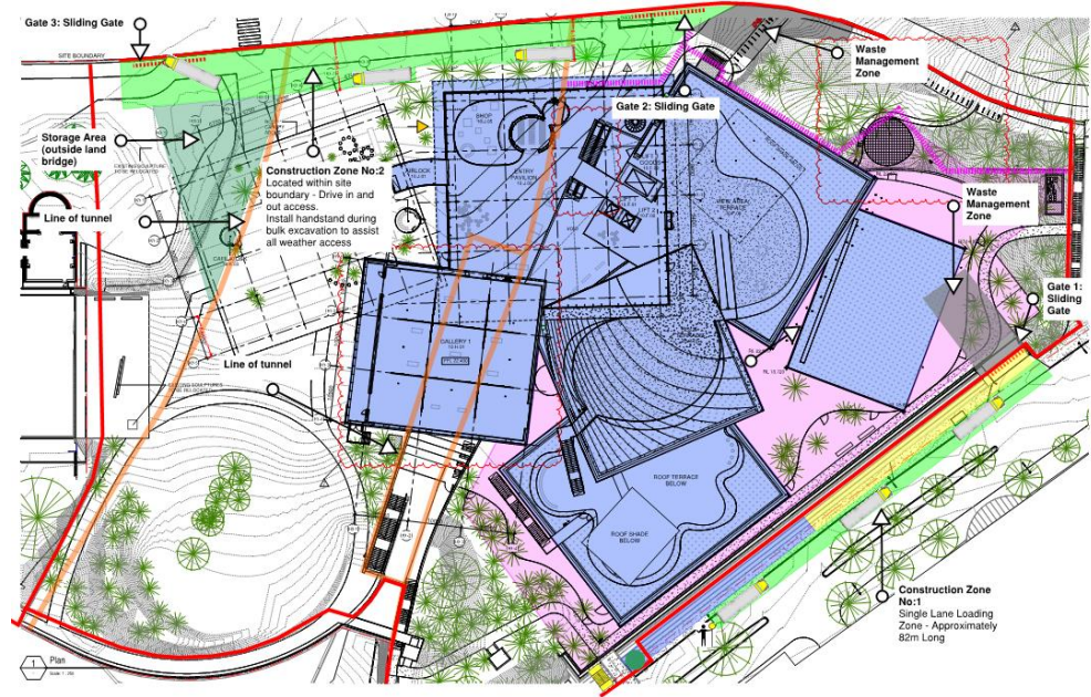
Site Plan - Construction Waste Management Zones
