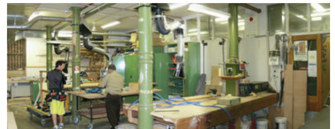
Workshops, Vernon Wing, LL1. The cast-iron columns are remains from the Walter Liberty Vernon design.
