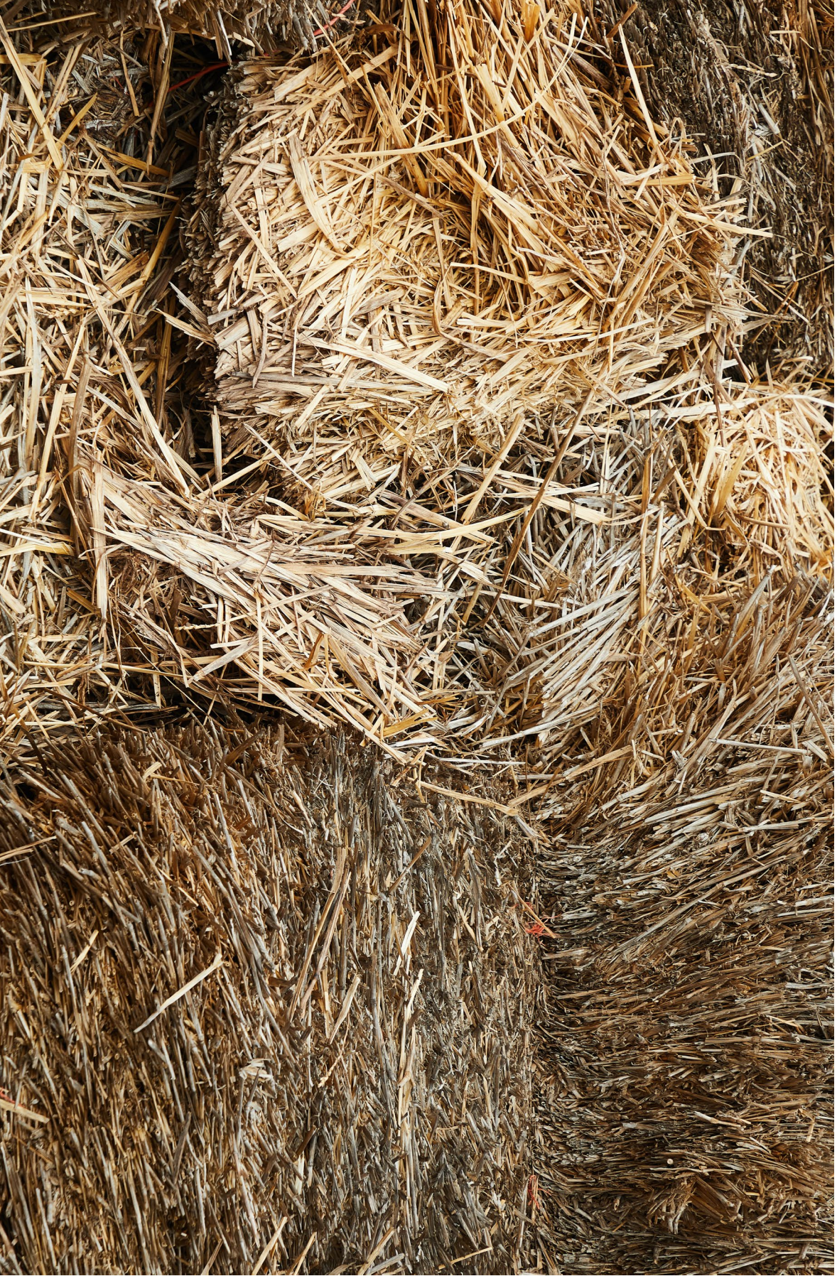
Straw bales: Straw bales are compressed and bound straw, typically wheat or rice straw. They are used as building blocks for walls, offering good insulation properties and contributing to energy-efficient construction.
