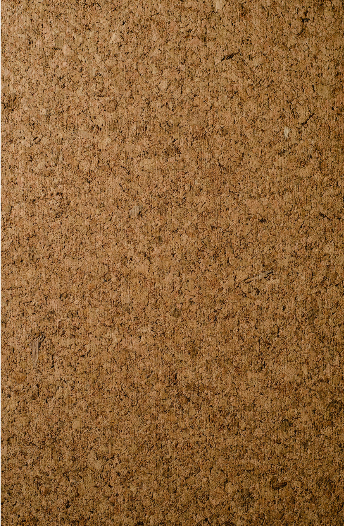
Cork: Cork is a natural material that is harvested from the bark of cork oaks. It is a light, strong and sustainable material that can be used for flooring, insulation and soundproofing.
