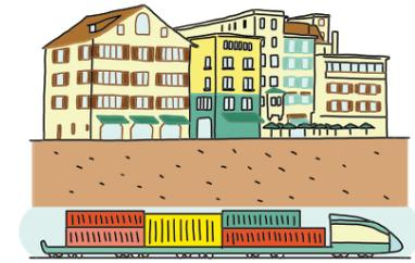
Containers will be conveyed through an underground tunnel at a speed of 30 km/h (18.6 mph) by automated vehicles powered by renewable electricity. Near their destination, usually in a city, goods will be unloaded in an underground hub then delivered to each address by light electrically powered vehicles, some of them driverless. The schedule and route for each delivery round will be calculated to ensure optimal efficiency.
