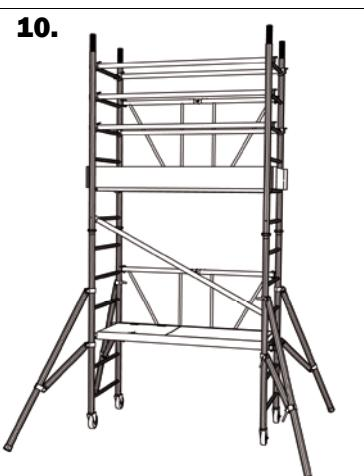
both fittings tight. The stabilizers should be put steady on the ground and the scaffold should stand vertically. (fig. 1 - 2 page 31)
