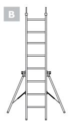
Every time the bottom ladder (B) is used, check that the stabilisers and leveller are locked.
