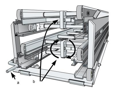
After use, slide the ladder sections into the correct rail in the mount until they are all properly in place.
