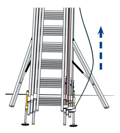
Release the ladder from the wall by lifting the ladder and lowering the stabilizers to act as a pivot.
