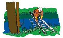
As a bridge with 2 ladder sections. Maximum load on a span of 4.5 metres = 170 kg.
