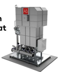
less impacting given their operation in "auto-thermal" mode. The RTO system can recover up to 96% of the latent heat of the purified gas and reuse it for preheating the inlet gas. This is done using a refractory material with a high heat transfer capacity. Operating temperatures range from 780 to 1,000 °C
