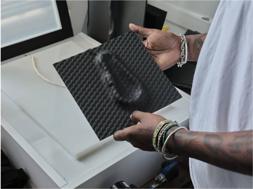
In the studio are a toaster oven and a vacuum press for making sculptures out of Kydex, a synthetic material used for gun cases. Hannah Price for The New York Times
