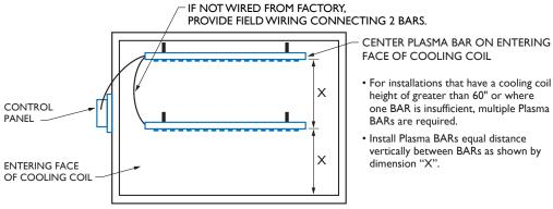
FIGURE Ic Plasma BAR Installation for Air Handlers Requiring Multiple BARs
