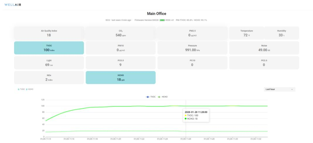
d. The **time range** of the trend graph can be adjusted using the **drop-down time selection menu**.
