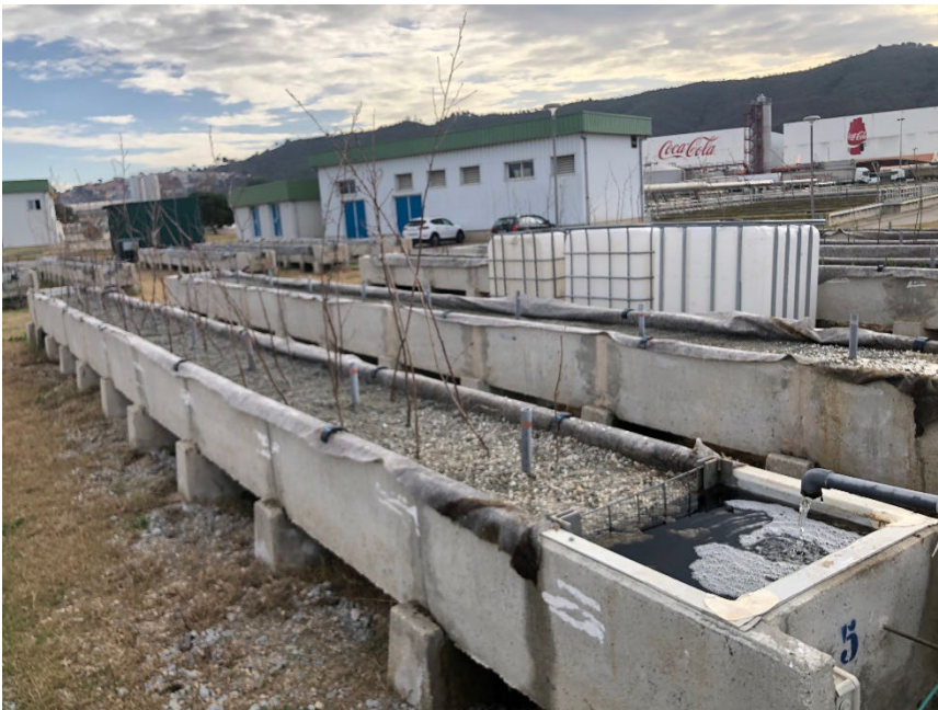
Figure 4. On the left, a scheme of a vegetated flume at the Urban River Lab experimental platform . This drawing shows the five PVC wells to collect the subsurface water through the substrate along the flume. On the right, panoramic picture of the flumes, which are fed with WWTP effluent of Montornès del Vallès (NE Barcelona)
