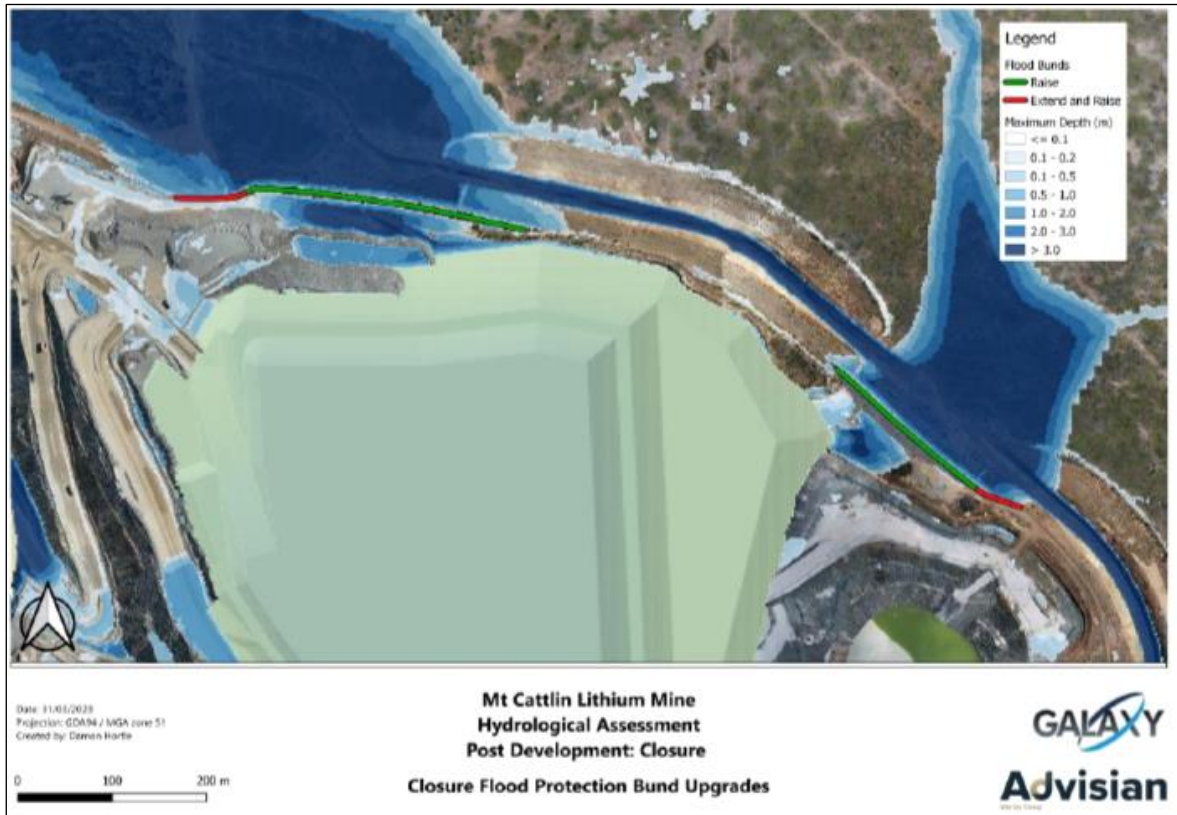
Figure 5-14 Locations Where Existing Flood Protection Bunds are to be Upgraded at Mine Closure (Advisian, 2023)
