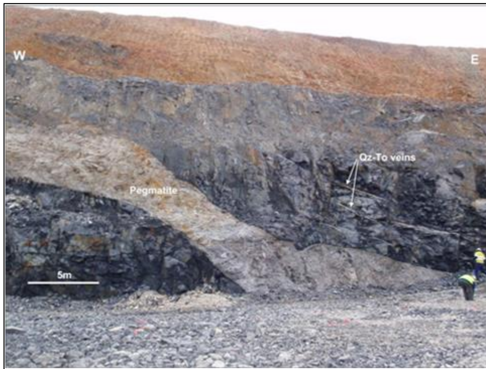
Figure 7-5 Mt Cattlin Pit 1A North Wall Showing Pegmatite and Quartz Tourmaline Veins
