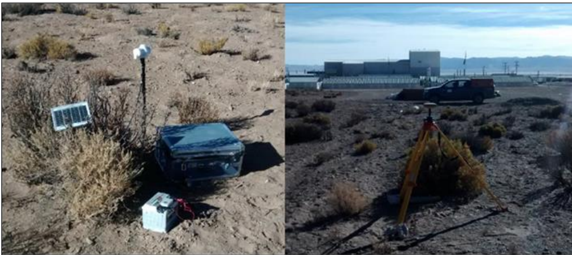
Figure 9-7 – Installation of the magnetic base station (left) and the GPS base station (right).
