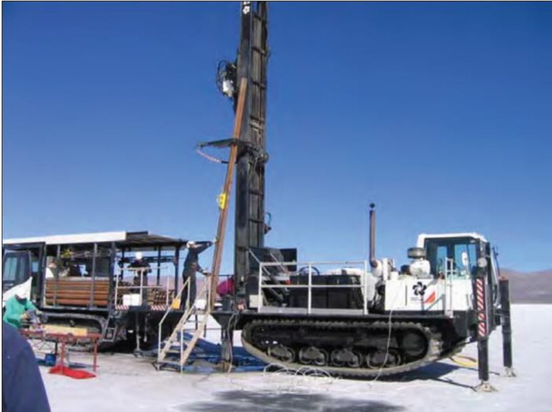
Figure 9-13 – Sonic drilling rig operating at Olaroz in 2010.
