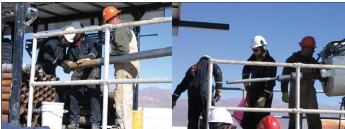
Figure 9-14 – Recovery of the lexan core and split spoon samples on the sonic.
