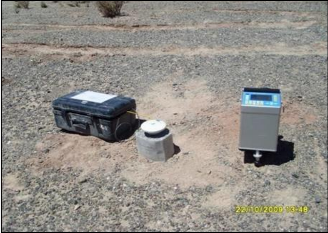
Figure 9-4 – Gravimeter base station.
