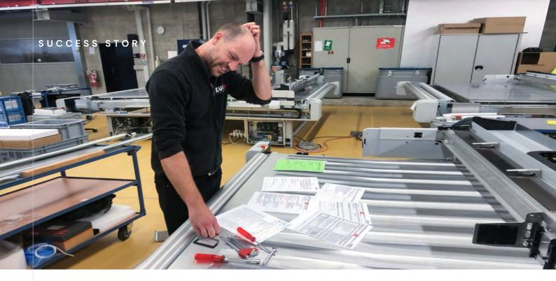
During the assembly of the vacuum table, the bars and the control unit, many measurement points 3 are made with regard to electrical safety, electrical cabling, positioning accuracy of the process, oscillation of the entire system, etc. If these settings are correct, the system is prepared for 4 dispatch.
