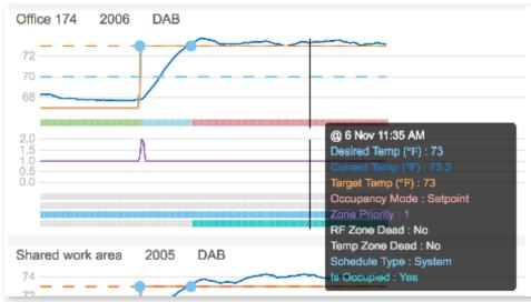
Facilisight<sup>®</sup> zone graph showing the system maximizing efficiency in unoccupied offices. When unoccupied, temperature is allowed to  $68^{\circ}F$  – then quickly adjusts to  $73^{\circ}F$  once occupied to match the desired setpoint.
