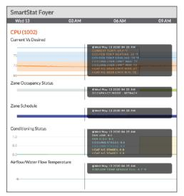
To see live datapoints such as zone temperature, humidity or airflow temperature, users need only hover their cursor over the zone. When Facilisight users click on the zone, they can also see all the user intent settings associated with that zone. Clicking on a system icon brings up parameters related to system or building operation. Some examples of this include minimum and maximum humidity settings, schedules, and vacation modes. These intents are editable from the same window.
