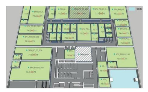
to maintain optimal temperature levels with higher energy efficiency levels. To measure improved energy efficiency, the 75F team installed energy meters and BTU meters at each AHU level. Energy meters have been installed at floor level and DB level to provide SMDB breaker-level energy management.
