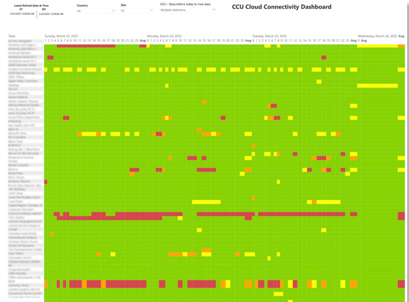
Gateway cloud connectivity using Wi-Fi networks. If Wi-Fi is ever down, 75F’s system automatically runs locally.
