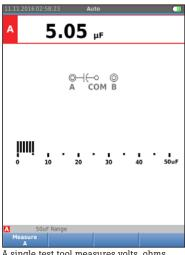
A single test tool measures volts, ohms, amps or capacitance, in addition to displaying waveforms.
