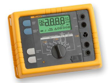
rod and each are connected to the tester. No earth ground stakes are used at all. A known, fixed voltage is induced by one clamp and the current is measured using the second clamp. Then the tester automatically determines the resistance of the earth ground rod.
