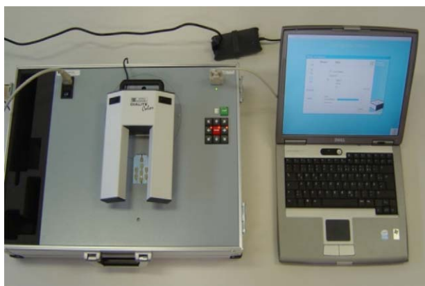
Fig. 2 – Toothguide Training Box (TTB) with the software support.
