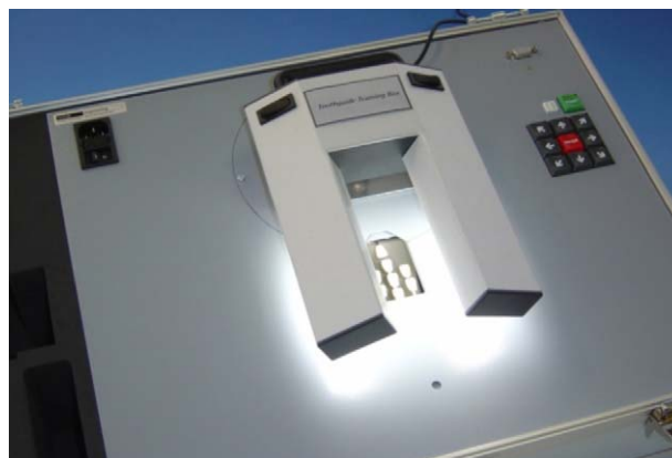
Fig. 3 – Toothguide Training Box (TTB) with the color corrected light source turned on.
