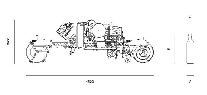
The line is designed on a customizable platform, with functionalities that can be added before and after installation, adding new features on the go. The composable nature of the machine allows expanding its capabilities to closely follow the company's growth. Components indicated with the symbol  $\triangleright$  cannot be removed.
