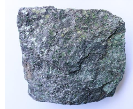
Balama graphite ore body with green bearing vanadium mica
