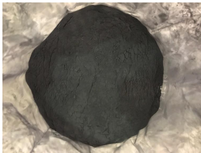
Milled spherical graphite for customer qualification
