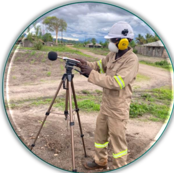
Noise monitoring being conducted in the Balama Village
