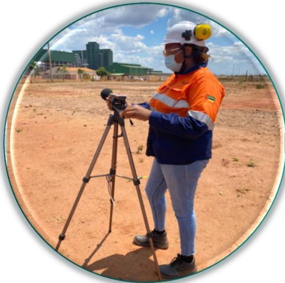
Noise monitoring being conducted at the plant site in Balama
