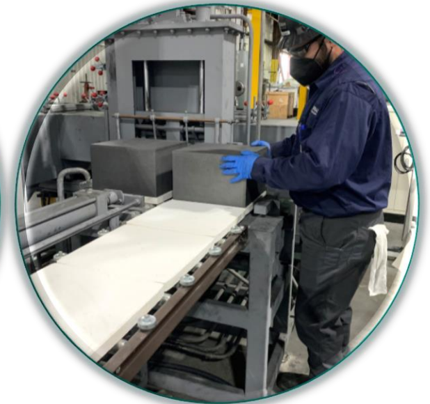
Employee loading raw material into the carbonisation furnace
