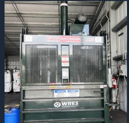
Baler machine for recycling super sacks used to transport graphite material
