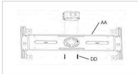
Attach the mounting plate to the junction box using the two screws provided. Align the mounting plate in the direction you want the fixture to be aligned. Once the toggle bolts are installed, you cannot change the orientation
