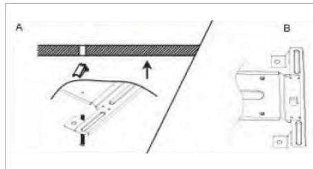
Feed the junction box wires through the center of the mounting bracket plate hole. Re-attach the mounting plate by inserting the four toggle bolts into the drilled holes. Once the wings are through and expanded, pull the screw downward to engage and tighten
