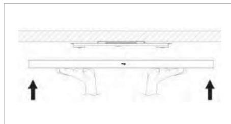
Put the mounting bracket into the panel light first, then aim the shrapnel on the back of the lamp, and put the panel light up
