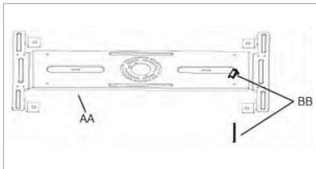
Remove the mounting plate from the junction box. Drill four holes where marked using a 1/2in drill bit. Remove the wings from the 3/16in toggle bolts. Insert a screw through the front of the mounting plate and reattach the wing to the screw. Repeat for all four toggle bolts
