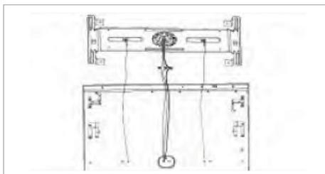
Connect the three wires coming from the fixture to the junction box wires
