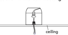
fig 2. Plug cable connector on adaptor into the downlight.
