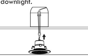
fig 3. Push the downlight to fit in the can housing.
