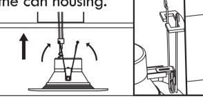
fig 4. Release clip arms and push the downlight into the can housing.
