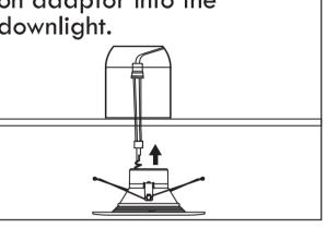
fig 3. Squeeze the spring clip arms up on both side and hook the clip arms into the arm hooks on the inside of the can housing.
