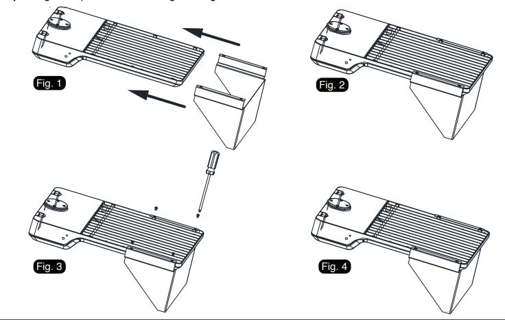
Step 1: Put the backlight shield on the fixture as Fig. 1 & Fig. 2
