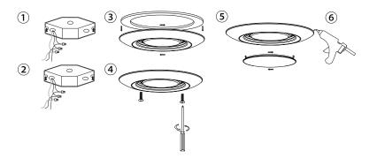
**STEP 1** Prior to installation. Please install two screws (furnished) into the junction box. Do not drive screws completely to the end of the junction box. **STEP 2** Connect supply wires to wires in fixture wiring box with proper size wire nuts or push wires into "push-in" connector. Connect white to white, black to black and green or bare copper wire to bare copper wire.
